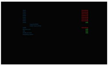
When an abnormality is detected and the self-test screen stays on, choose to continue or shut down in the lower right corner of the screen. If you choose to continue, the NVR enters the login interface.
