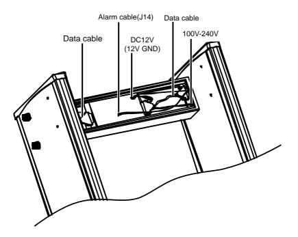
5. Close the rear cover plate on the control unit and use the supplied bolts to secure the control unit and the crosspiece.
