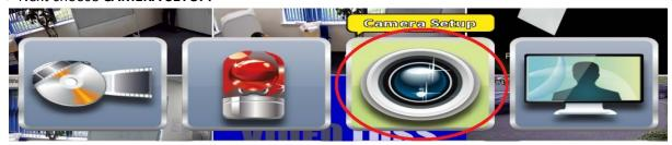
> In **CAMERA SETUP** select which channel the PTZ is connected to (1) then enable **RS-485** (2). You will now be able to edit the **Protocol**, **PTZ ID** and **Baud Rate**.
