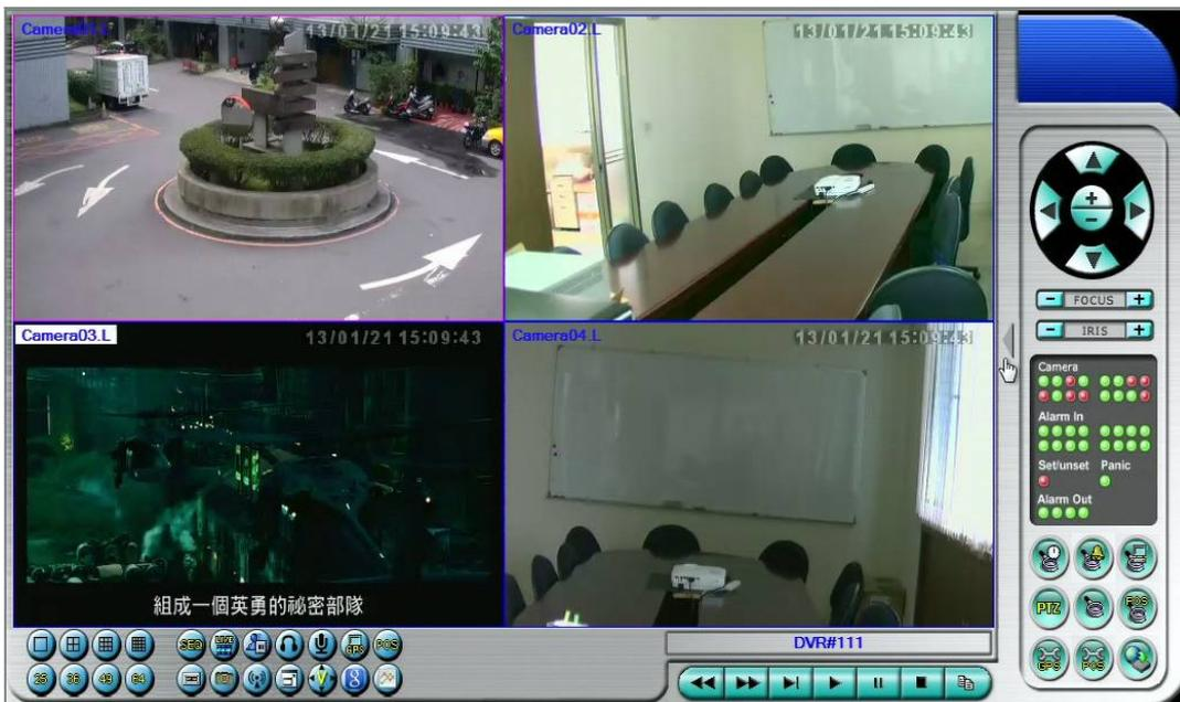
The video images can be displayed in several types of split-window screens, including 1/4/9/16-Window for single DVR and 25/36/49/64 for multiple DVRs. And the focus window is surrounded by a frame border. In addition to the video windows, there are different icons on the lower corner and the right corner of the screen for status display and control. (The “.L” following the camera title stands for Live display, “.P” for Playback, and the camera title with white background has detected motion.)
