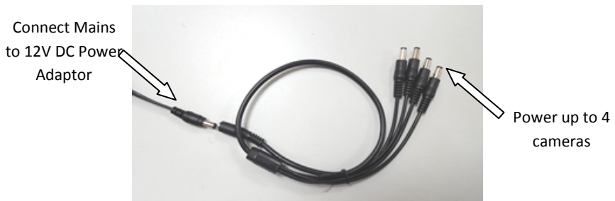
Using DC 1 to 4 Y cable to power up to 4 cameras from 1 power adaptor
